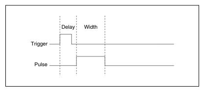
Figure 4-2. High Pulse with Rising Edge Trigger
